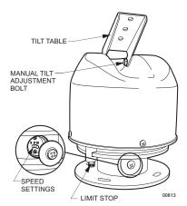
Figure 4. Scanner Adjustments and Settings
